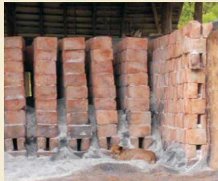
Photos from improved brick production workshops in Badulla district depicting: Improved stacking in the drying process; kiln introduced by the project; improved brick stacking for the firing process.
