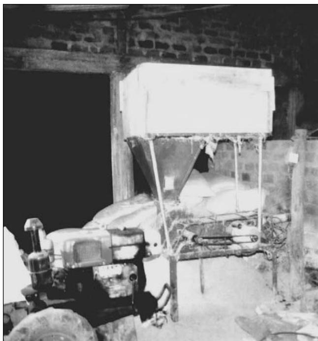
**Motor for improved bakery oven using rice paddy husk as fuel (Sri Lanka).**
